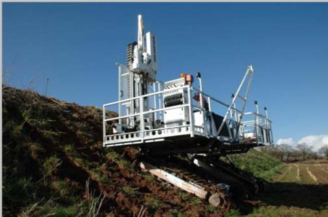
One of our well known innovations, the **Pioneer rig**, is a small, track mounted unit, which has the ability to dynamic sample in soft ground and core in rock. This multi-functional rig has proved very popular due to its compact footprint and continuous sampling capability.
