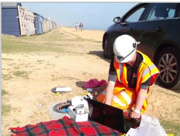
We carry out a range of tests in accordance with BS1377 including plate bearing tests, in situ CBRs, sand replacement density testing and thermal and electrical resistivity measurements. We also offer dynamic cone penetrometer testing.
